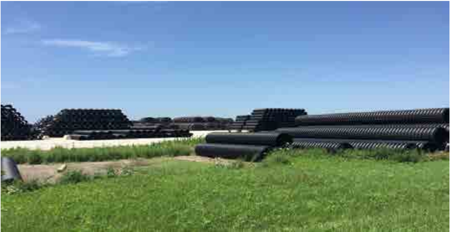
A green area with multiple piles of black plastic drainage pipes scattered. The sky is blue and the sun is out. HDPE drainage pipe outside., Chardsworth, IL.
